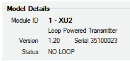
If the transmitter does not have the correct software installed, the following will be shown:
