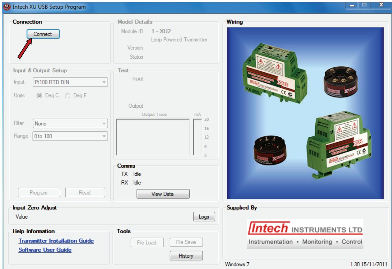
Connect the XU transmitter to the USB plug and click Connect. Wait for the software to establish a connection.
