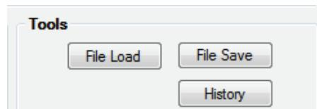
Click File Load to load a txcal file into the TX.
