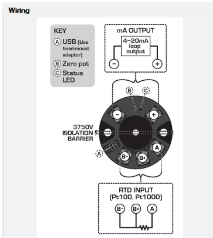
This panel shows the connections to the Transmitter required for the input type selected.
