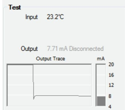
Shows a panel giving current input and output value, and a short duration trend graph of the output. This panel will show a live input reading when the transmitter is only powered by the USB connection.
