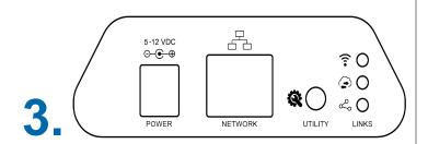
Connect the antenna and ethernet cord. Then attach the power cord to your Ethernet Gateway 4. All lights should turn green.
