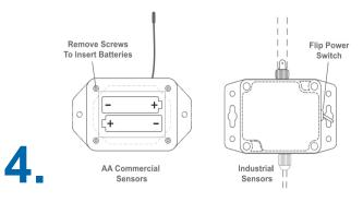
Insert batteries or use the switch to power on the wireless sensors.
