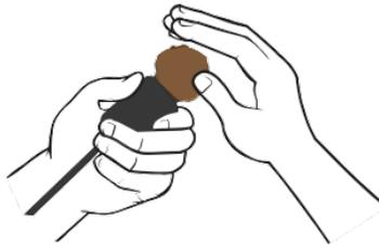
**Note:** Sandy soils may not adhere to the sensor even when wet. If so, place the sensor at the bottom of the hole and carefully pack the soil around the sensor. Be sure to pack the soil firmly around ceramic surfaces.
