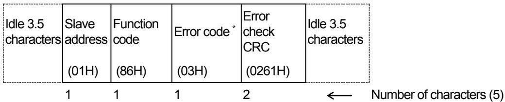
In a response message during occurrence of an error, “1” is set to the MSB of the function code (86H). An error code 03H (value outside of setting range) is returned as the response message for the error content.
