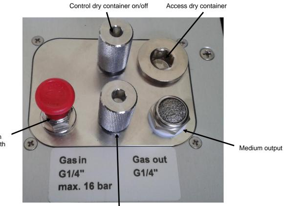
Plug in connection Medium closed with red seal plug.
