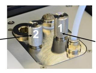
Control Medium (1) open, max. until red marking is visible
