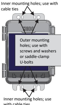
**Important:** See the RX2100 manual for additional deployment guidelines at [www.onsetcomp.com/resources/documentation/23808-rx2100-manual](http://www.onsetcomp.com/resources/documentation/23808-rx2100-manual).
