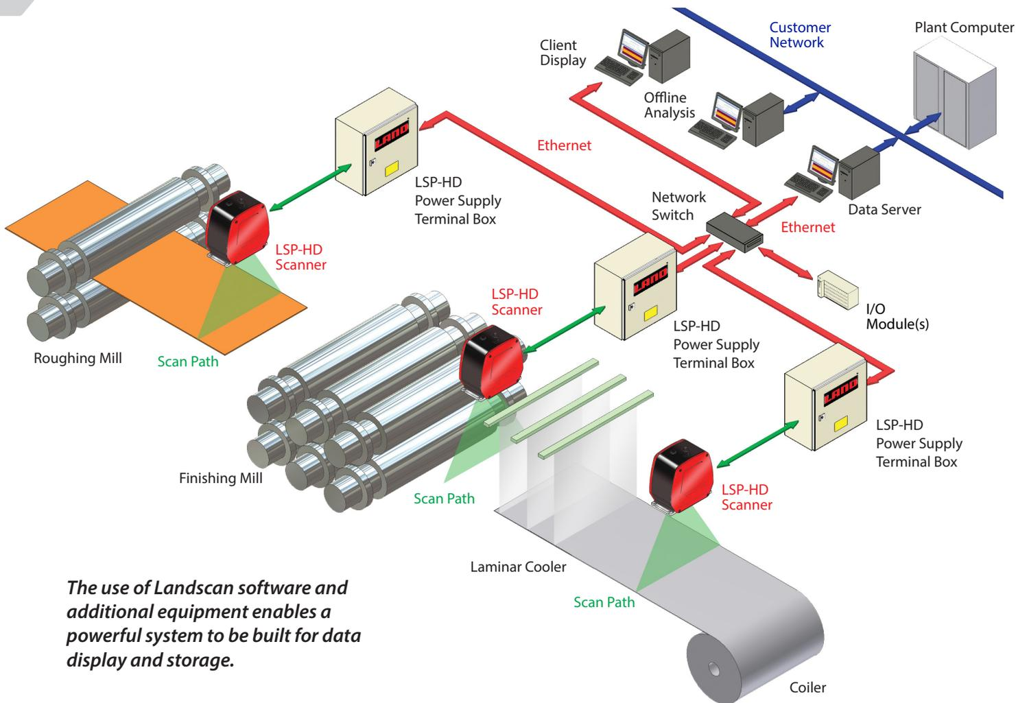
*The use of Landscan software and additional equipment enables a powerful system to be built for data display and storage.*
