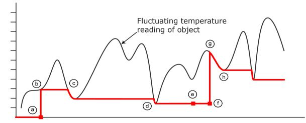
Fig. 7-4 Graphical representation of typical **Valley** temperature measurement
