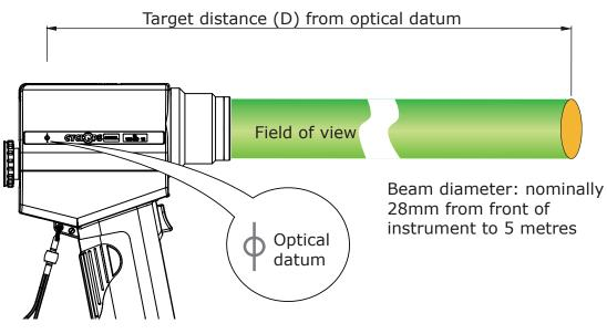
Fig. 6-2 Cyclops 055L thermometer field of view
