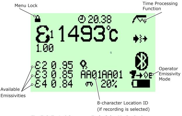
Fig. 7-6 Typical Operator Emissivity Mode display
