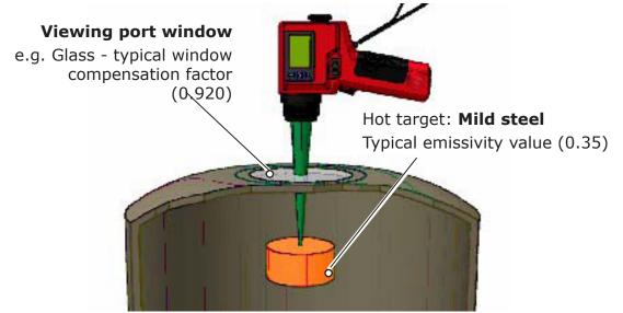
Fig. 9-1 Typical complex temperature measurement application
