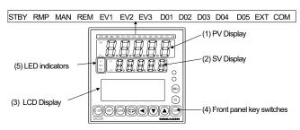
The front view is an example of the basic function SS. (Differs from the basic function MS.)
