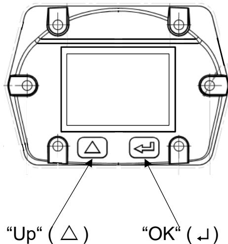
The operation of the VA 500 is done by the two capacitive key buttons Up ( $\triangle$ ) und Enter ( $\leftrightarrow$ )
