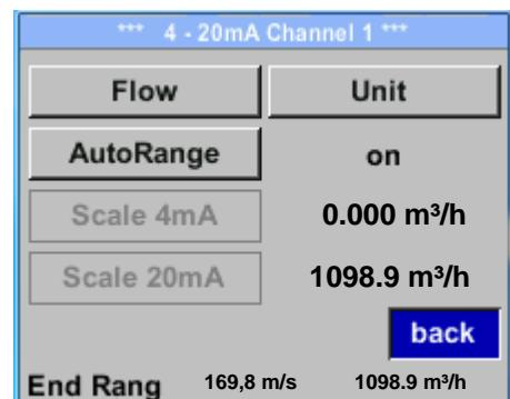
The 4-20 mA Analogue output of the Sensor VA 500 can be individually adjusted.
