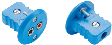
Type T ANSI illustrated (R32T-A). Cutout diameter = 28.3mm
