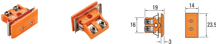
Type N ANSI illustrated (F29SN-A). Recommended cutout: 8mm x 16.5mm
