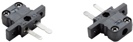
Type J ANSI illustrated (F37J-A). Recommended cutout: 8.5mm x 16.5mm
