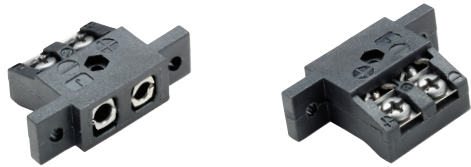
Type J ANSI illustrated (R27J-A). Recommended cutout: 13mm x 26mm
