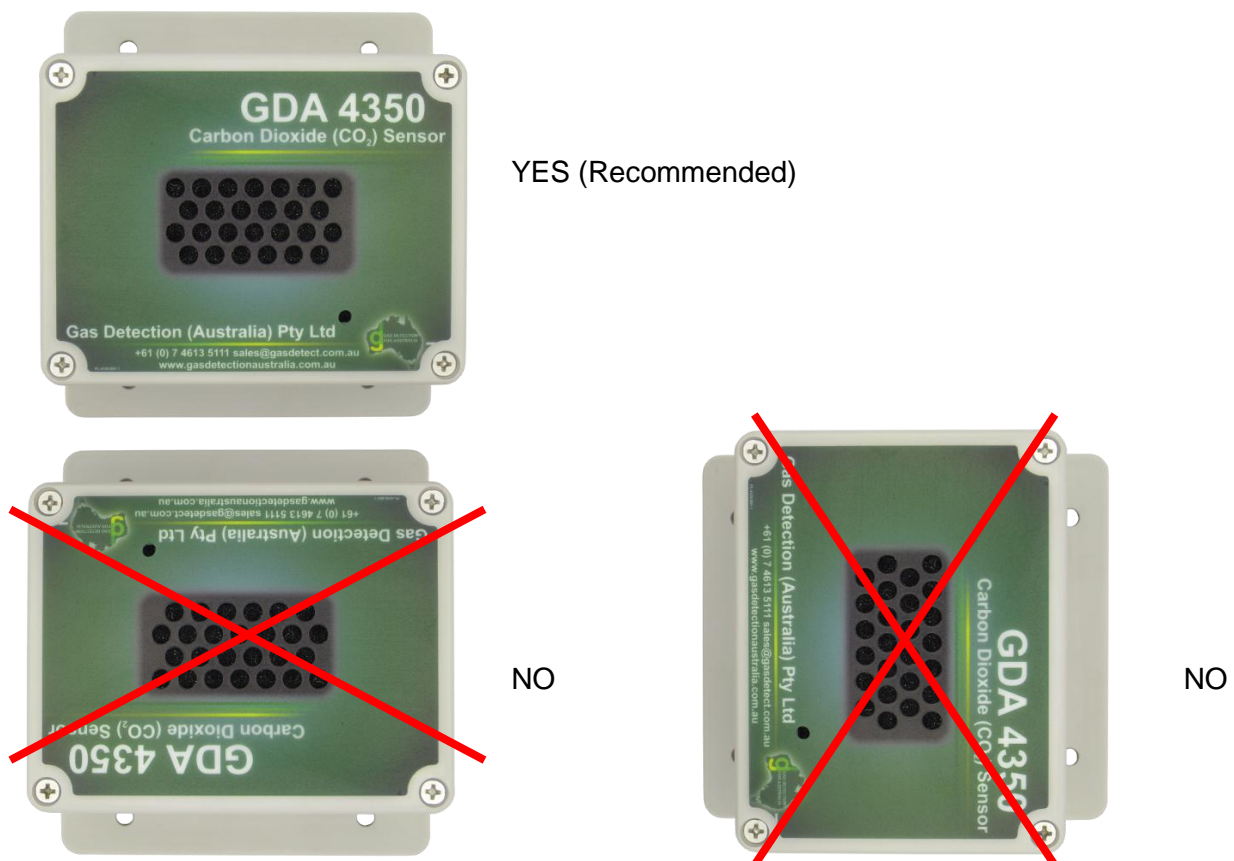
Figure 2: Sensor Mounting orientations
