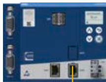
JUMO variTRON 500 Central processing unit for an automation system Type 705002
