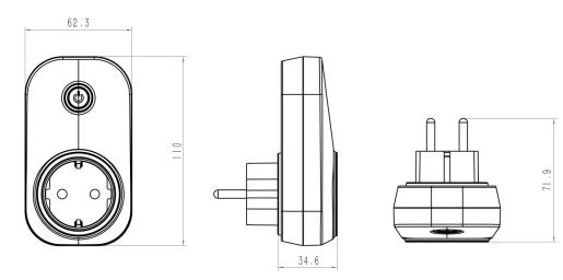
Note: The plug size will a little differ according to socket types.
