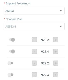
If device frequency is one of CN470/AU915/US915, you can enter the index of the channel that you want to enable in the input box, making them separated by commas. **Examples:**
