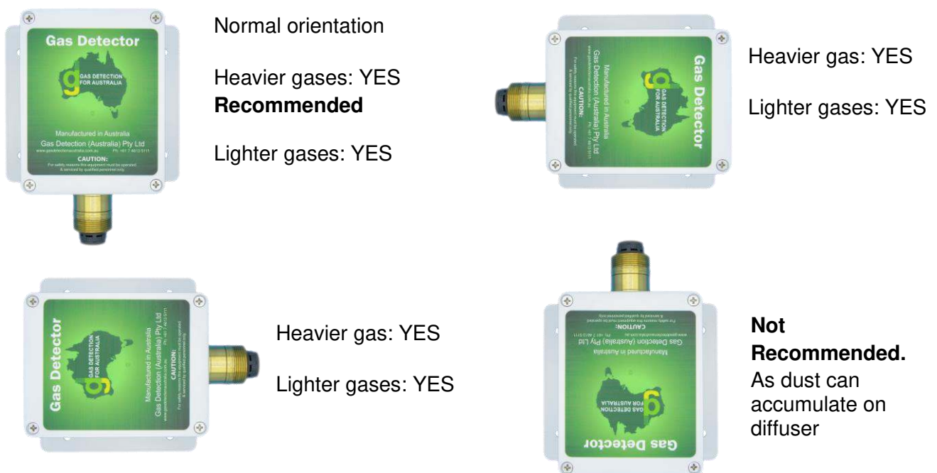
Figure 3: Sensor mounting orientation.
