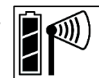
Once the mote has finished joining the network, the "x" icon is removed and the channel count on the station LCD increases by two (one for leaf wetness and one for the mote battery).
