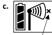
This network connection "x" icon blinks while the mote completes the registration process, which may take up to five minutes.
