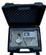
Compressed air quality measurement
